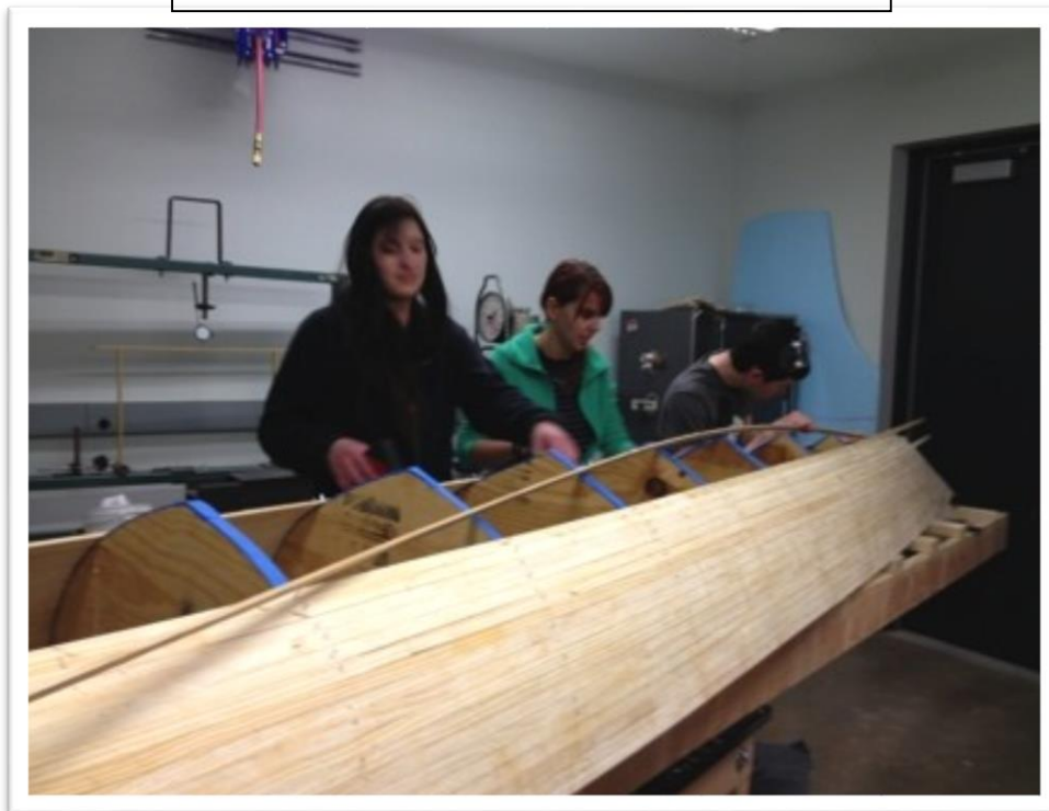
Photo 4: Attaching Wood Strips to Cross-
